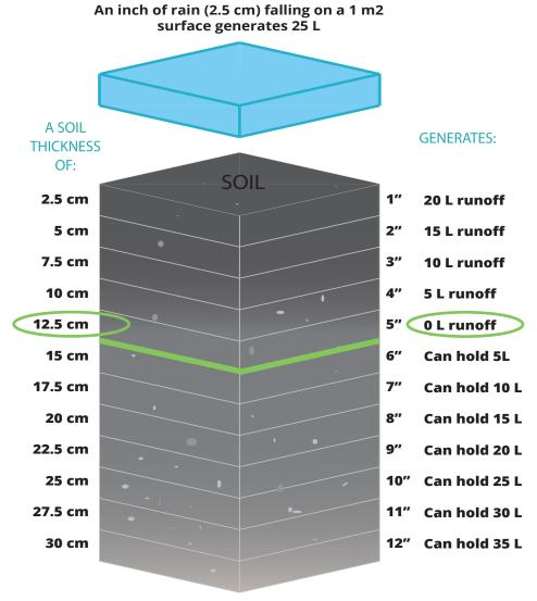
Soil has 20% open space. To fully hold this 2.5 cm of rainfall, it will take 12.5 cm of soil depth. If you have deeper soil, you have added capacity to absorb flows from other hard surfaces on top of what occurs naturally: An added 5 L per every 2.5 cm of soil depth per m2. This is a great approach for new development or slopes where you can add soil as terraces.
